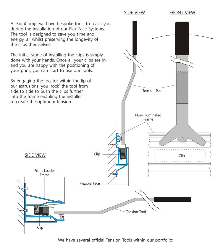
Our 5135 is designed for our Econoflex and Retro Frames. The 5137 is used with our Non-Illuminated and Front Loader Frames. Our 5138 is specially designed for our Non-Illuminated where there is limited access around the frame.
