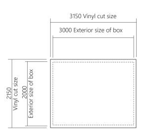
Add 150mm to the height and width (75mm on each side) of the finished size of the frame #7000 ie. For a frame that has overall measurements of 3000 x 2000mm, the vinyl should measure 3150 x 2150mm.
