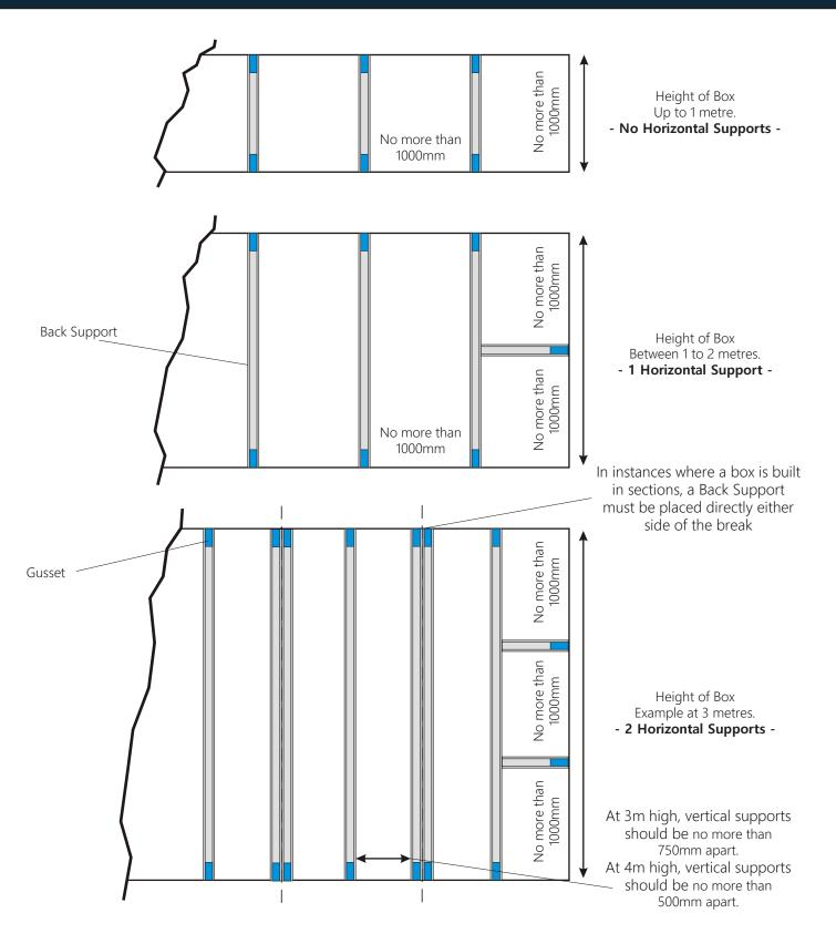
Both Vertical and Horizontal Back Supports cannot be more than 1m apart in any size box. When your boxes are larger, you should move the supports closer together to account for the additional weight and print size When calculating section sizes, please factor in your transport to site and the installation process This is just a general guide and every project needs to be looked at in isolation. Contact us for more advice -
