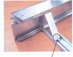
Drill and rivet / (Weld if equipment is available)
