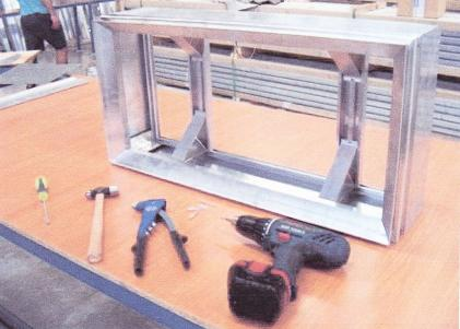
Once the sides have been finished the covers (#7200 or #7300) can be fitted and the box can be painted. The box can now have its aluminium backing sheet and the electrics fitted.
