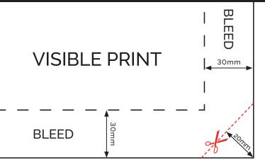
We recommend trimming the corners for ease of installation, removal of prints and to ensure the longevity of the internal Grip Strip is preserved. Installing too much fabric into the frame may result in damaging the Grip Strip upon removal. Cut the corners at a 45° angle up to 20mm into the print.
