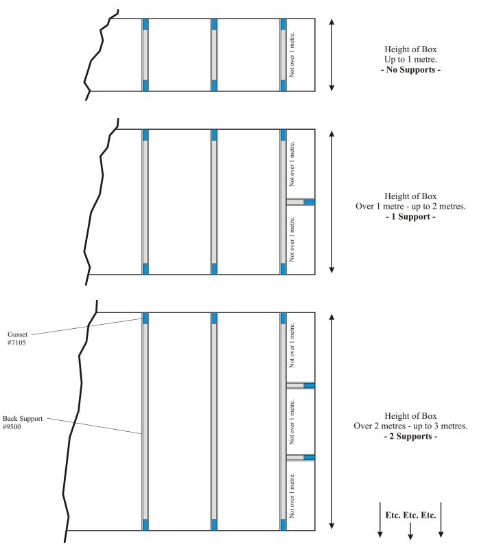
Signs that are 3 to 3.5 metres close the back support in to 900mm centres Signs that are 3.5 to 4 metres close the back supports in to 800mm centres Signs that are 4 to 5 metre close back supports in to 700mm centres above these heights please check with SignComp for their recommendation.
