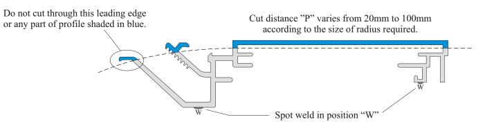
**STEP 1 - CUT FRAME** (Pitch "P" dependant on required radius "R")
