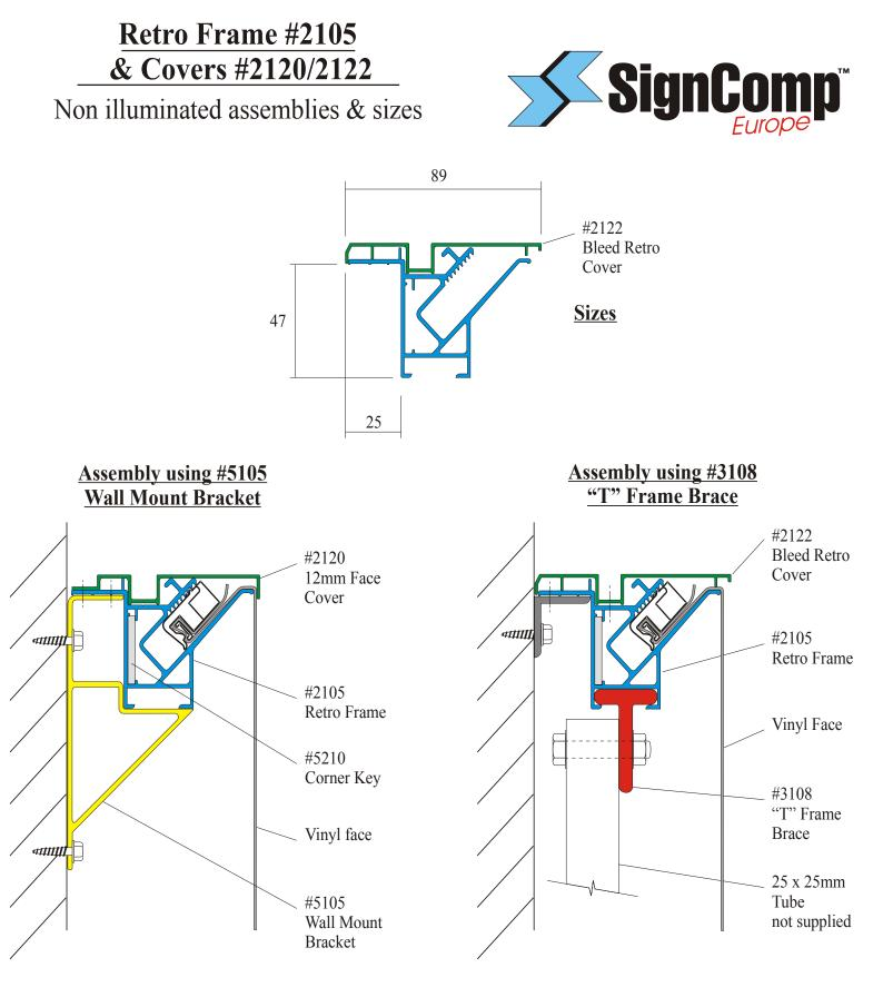
Place the #5105 Wall Mount Bracket or the #3108 "T" Frame Brace on maximum 1000mm centres. Where frames join, a #5105 Wall Mount Bracket should be placed each side of the frame joint. (For signs of more than 4000mm in height, reduce spacing to 600mm)
