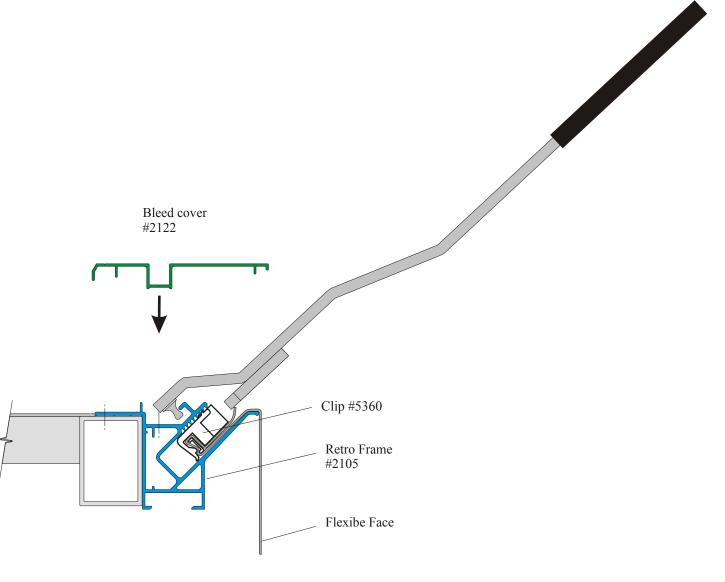
When tension tool is in position, move from side to side over the clip to press the clip down.
